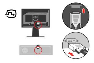
Connect the analog signal cable to the D-SUB connector of the monitor and the other end on the back of the computer.
